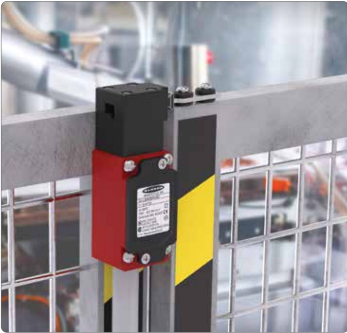
Mechanical switch on large gate
